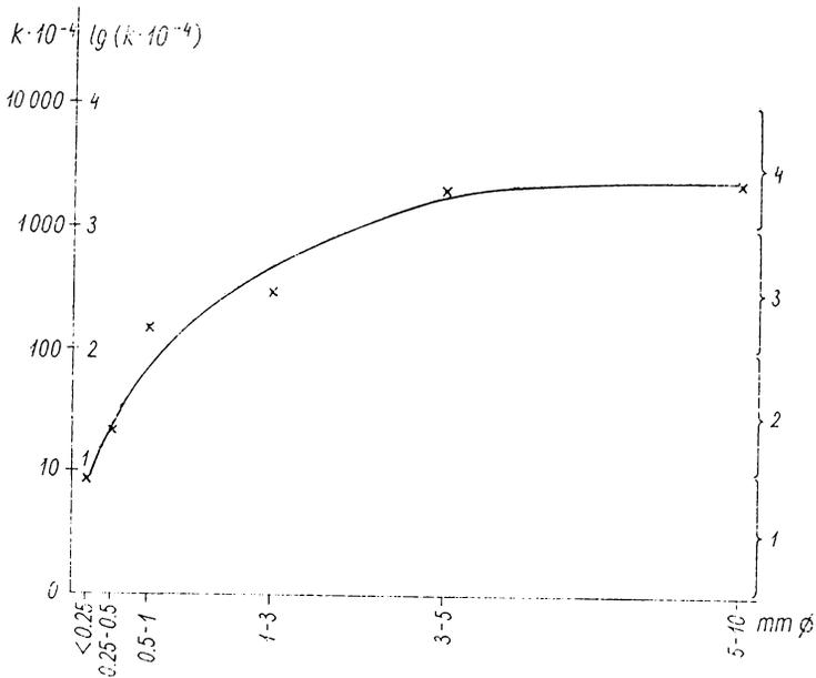
Fig. 1. Water permeability coefficient value for aggregates of different size and ranges of water permeability coefficient values for different formations after Hillel
