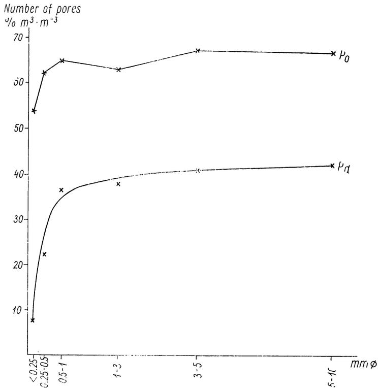
Fig. 2. Relationship between the size of aggregates on the one hand and the total porosity ( $P_0$ ) and the number of large pores ( $P_a$ ) on the other
