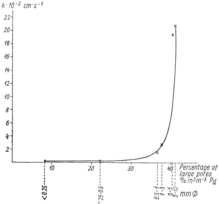
Fig. 3. Relationship between the water permeability coefficient value and the number of large pores in soil samples of different size of aggregates
